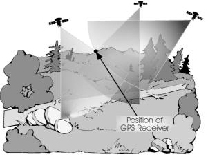
Measurement from 3 satellites (2-Dimension Navigation) gives an horizontal resolution of 10-20 meters and vertical resolution of 20-80 meters. Measuring signal from 4 satellites we are obtaining 3-D resolution. More satellites for simultanious measurement increses the resolution of the system. Testing Garmin GPS 12 I was checking 9 satellites (quite typical for Europe) I was obtaining EPE (Estimated Precision Error) of 3m resolution and making long-term measurements with resolution of 10m.
